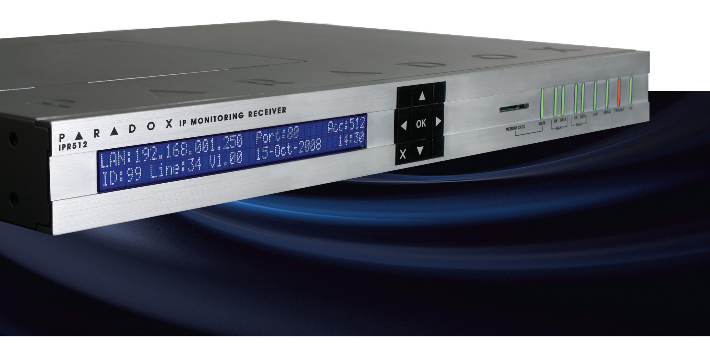
Up to 1024 supervised Paradox control panels can report system events to the IPR512 receiver over an IP network via a Paradox GPRS / IP reporting module (PCS Series Modules / Internet Modules ). All this is achieved through proprietary encrypted communication between the control panel, the Paradox reporting module and the IPR512 receiver. The IPR512 receiver also supervises the automation software and all 1024 connections (control panel presence and IP communication) at a configurable rate.
